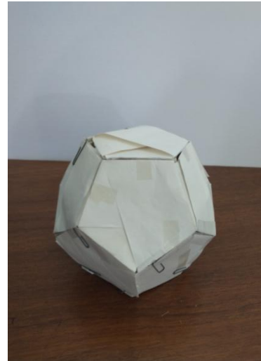
Figure 7. The 14 continuous pentagon spiral-enfolded dodecahedron
