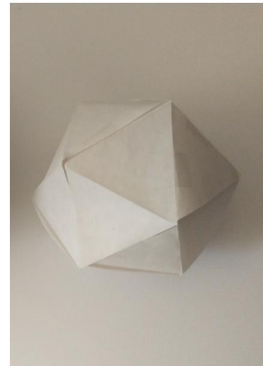
Figure 8. The 20 continuous triangle circular-folded icosahedron
